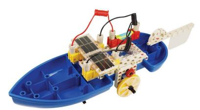
You will build a boat that will be powered by the sun. You will learn how to calculate the energy going into the boat through the solar panel and the efficiency of the system.
